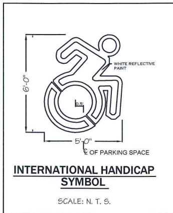
HANDICAP PARKING SIGN DETAIL SCALE: N.T.S.
