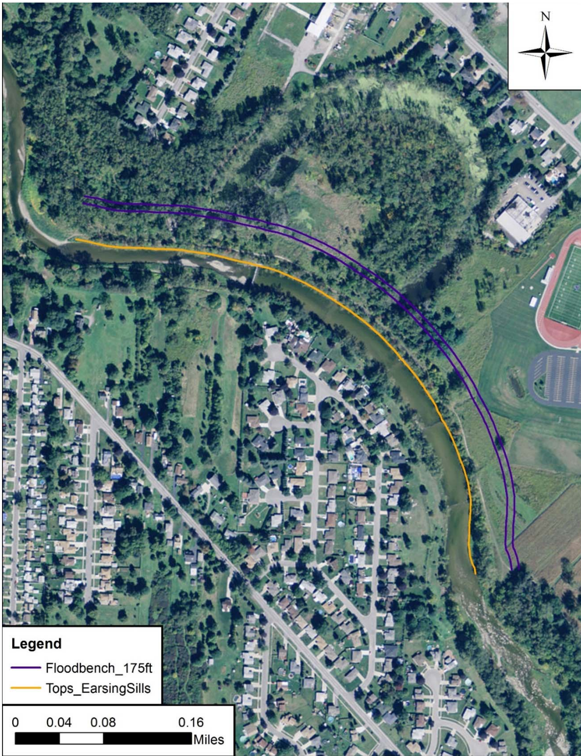
Figure 8: Measure 2 Flood Bench (210 feet wide, 3,060 feet long)
